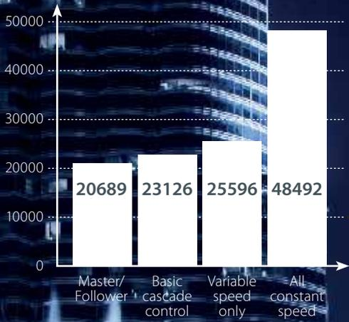
Using Master/Follower mode can reduce the energy consumption to less than half compared to traditional technology across the line for on/off cycling of pumps or blowers, and valve throttling.
